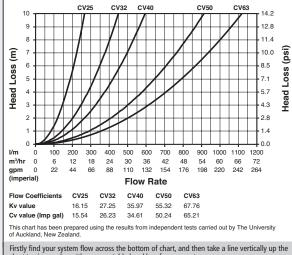
chart to size a valve with an acceptable head loss for your system.
