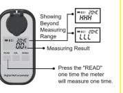
If press the "Read" button for 2 seconds, the instrument would make the automatic measurements upon programmed times (default 15times), the final value is the average of 15 times' measurements. After measurements, the multi-functions display area would return back to scale showing status.
