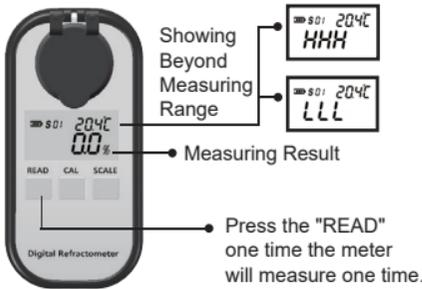
If press the "Read" button for 2 seconds, the instrument would make the automatic measurements upon programmed times (default 15times), the final value is the average of 15 times' measurements. After measurements, the multi-functions display area would return back to scale showing status.
