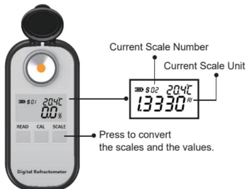
6.2 Temperature System Converting
