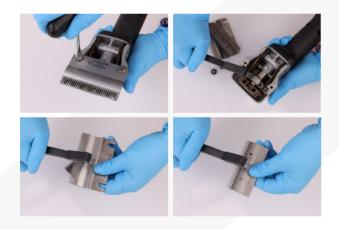
Simply unscrew the clipper blades from the cutterhead using the supplied screwdriver. Use a soft brush to delicately cleanse both the blade's teeth and the housing. After cleaning, reattach the blades, ensuring the screws are securely fastened, and employ the torque key to guarantee proper tension.
