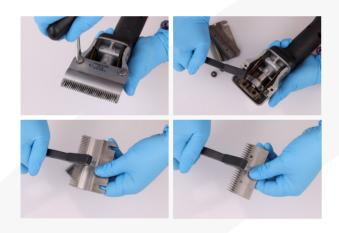
Simply unscrew the clipper blades from the cutterhead using the supplied screwdriver. Use a soft brush to delicately cleanse both the blade's teeth and the housing. After cleaning, reattach the blades, ensuring the screws are securely fastened, and employ the torque key to guarantee proper tension.
