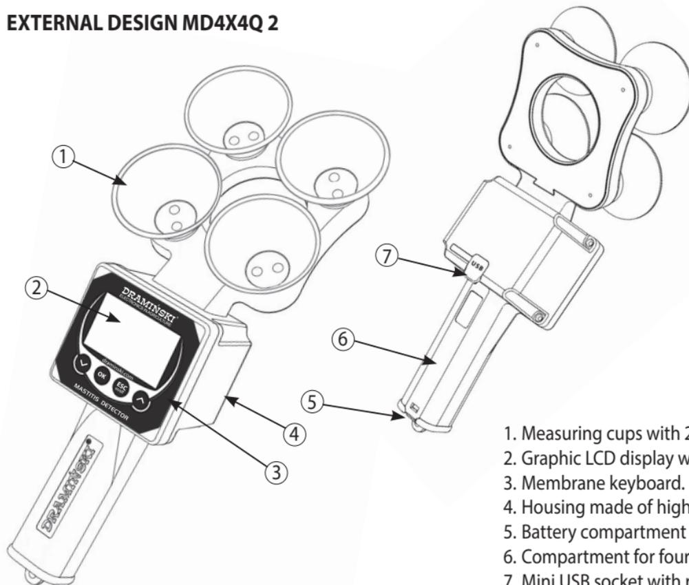
1. Measuring cups with 2 electrodes at the bottom.
