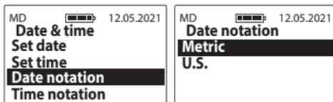
5.6 d) **Time notation** – to change the format of time display, go to **Main menu / Settings / Date & time / Time notation**, then use the or key to select the appropriate option and confirm with the key, e.g.
