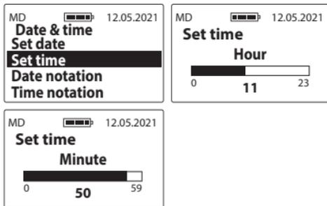
5.6 c) **Date notation** – to change the format of date display, go to **Main menu / Settings / Date & time / Date notation**, then use the or key to select the appropriate option and confirm with the key, e.g.
