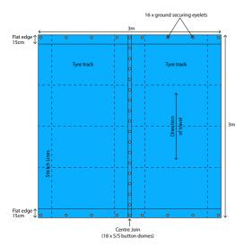
The vehicle mat is manufactured from marine grade thread, bonded-urethane foam core and a permeable, heavy-duty geotextile that enables disinfection of tyres as they pass over the vehicle mat. The amount of organic matter that can penetrate the vehicle mat surface is significantly reduced so there is little chance of the solution being neutralised and concentration rates are maintained for longer.
