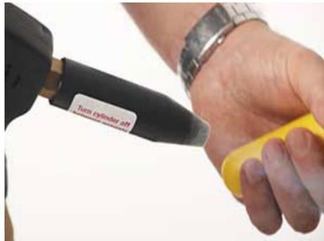
**DO NOT POKE ANYTHING METAL INTO THE JET** as it may damage the aperture, affecting the performance of the gun. Occasionally a cylinder of CO2 can have accumulated debris at the bottom causing partial or complete blockages. If this happens, we recommend contacting your gas supplier and having the cylinder replaced.
