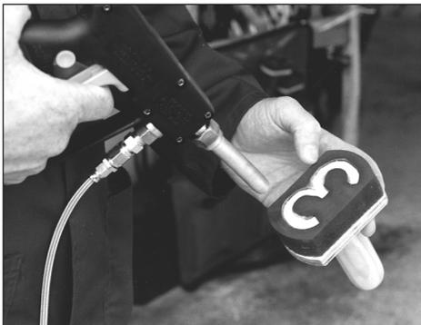
*Load the brand mould by holding the gun at right angles to the face of the brand.*
