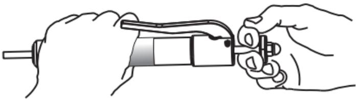
1. Clasp the device firmly with one hand in the handle area **[5]**.
