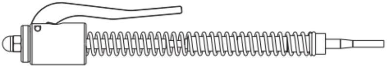
As soon as the spring has become shorter or the stunning result is no longer sufficient, the spring must be replaced.
