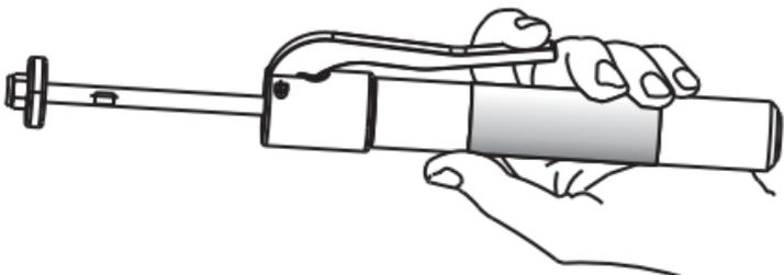
1. Hold the device in one hand so that your index finger can pull the trigger lever **[4]**.
